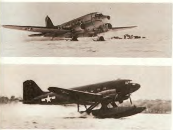
"Equipped with very large floats with retractable wheels, the C-47 became an amphibian (XC-47C); and on skis, it served in both the Arctic and Antarctic."
