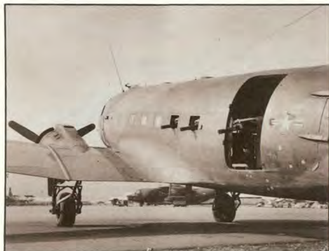
"Puff the Magic Dragon," the name given the AC-47D, had three General Electric 7.62mm Miniguns. At 6,000 rounds per minute per gun, each attack Gooney could pulverize a target and could loiter over a target area for hours.
